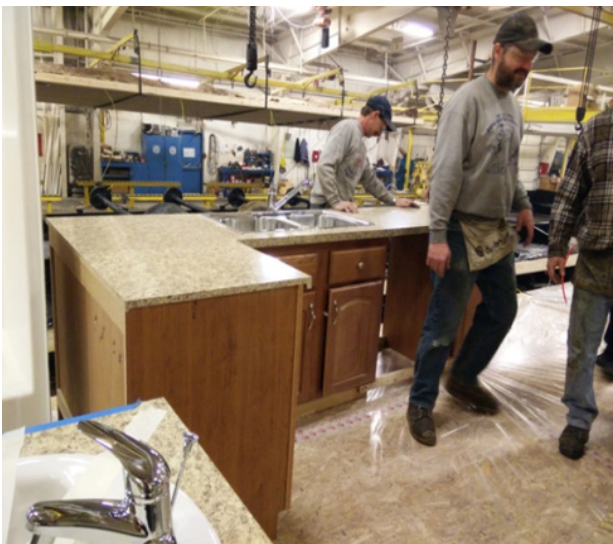
Figure C-15. Kitchen cabinets are placed on floor early in production process
