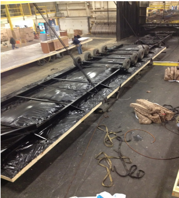
Figure C-9. Completed floor assembly before flipping
